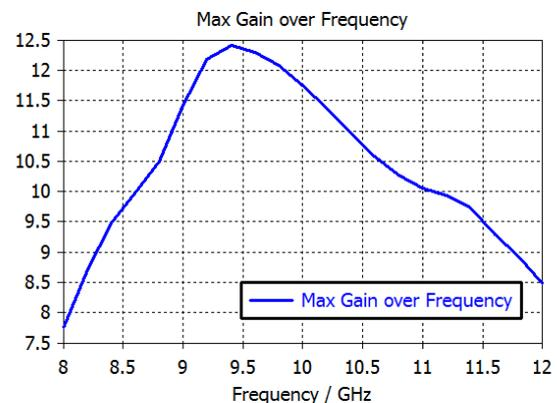
Fig. 8 Frequency characteristics of directive gain.
