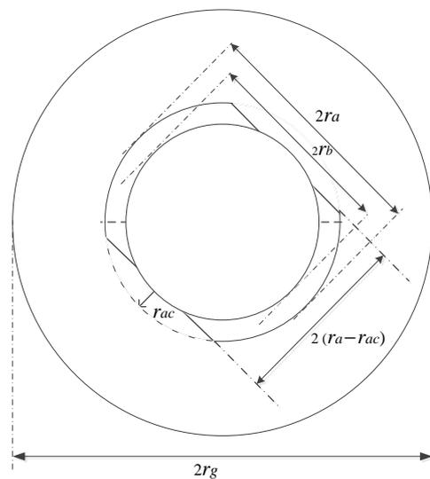
Fig. 2 Overhead view of the proposed antenna. The dimension of reactance element is included.
