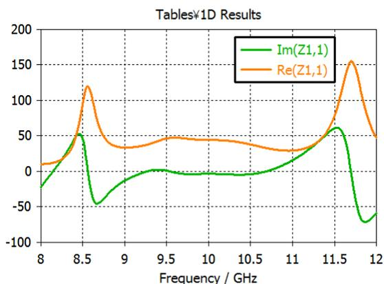
Fig. 9 Frequency characteristics of input impedance. Upper line: the real part of impedance. Below line: the real part of impedance.
