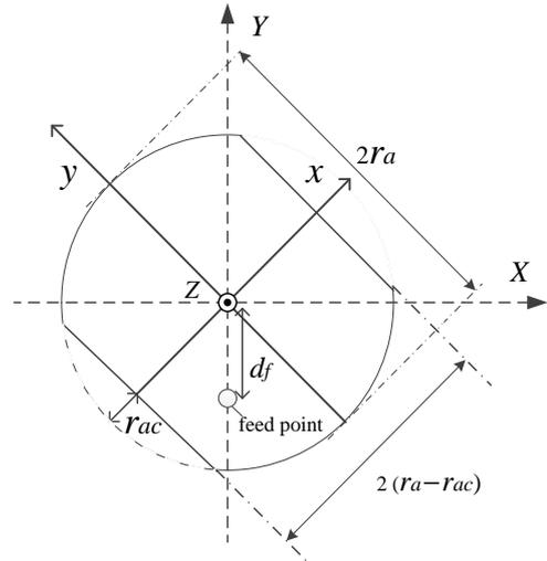
Fig. 4 Dimension of feeding element.
