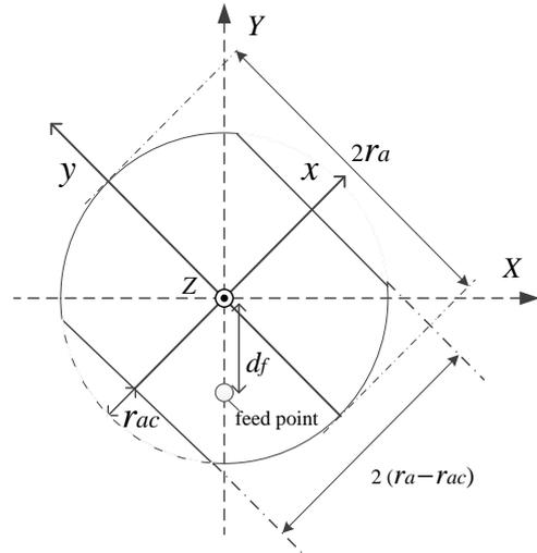
Fig. 4 Dimension of feeding element.
