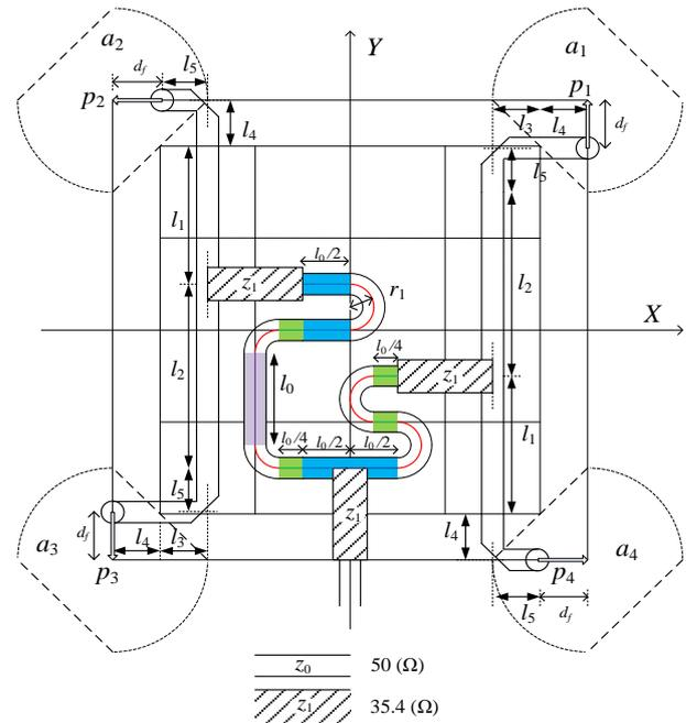
Fig. 6 Routing wire pattern for the proposed array antenna with 4 unit antennas.
