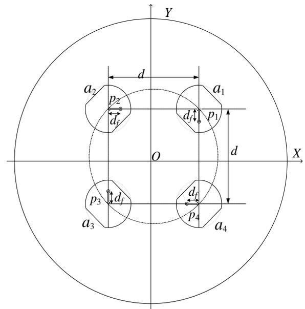
Fig. 5 Configuration of plane array antenna. Reactance elements (patches) and dielectric substrate are abbreviated.
