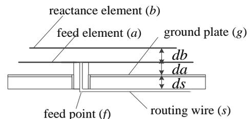
Fig. 3 Cross-sectional view of the proposed antenna.
