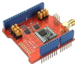
Figure 5: SX127x LoRa Shield
