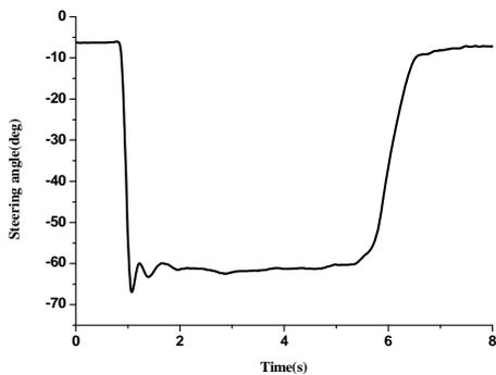
Fig. 7 The step input of steering angle
