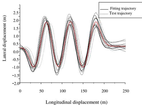
Fig. 15 the fit trajectory and the measured trajectory of slalom test
