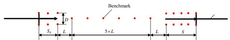
Fig. 13 the site layout of slalom test
