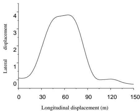
Fig. 18 the trajectory of double lane change test
