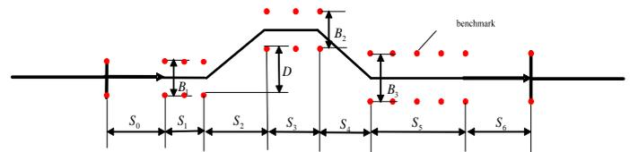
Fig. 12 the site layout of double-lane change test
