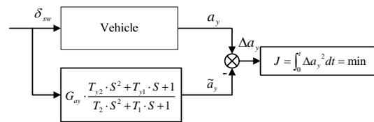
Fig. 4 the identification process of vehicle parameters
