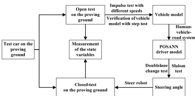
Fig. 11 the measure process of handling stability test
