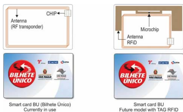
Figure 3 - Smart card with RF technology currently in use and a proposed the hybrid smart card with components of RFID technology.
