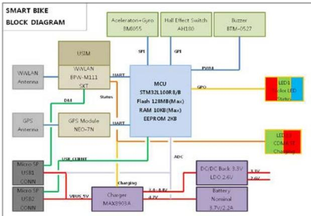
Fig. 1. Block diagram of smart device
