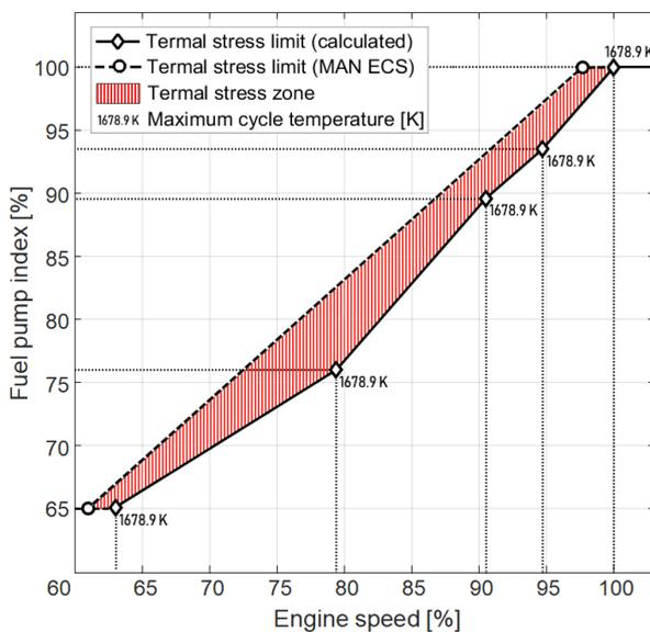
**Fig. 1.** The used and calculated limiting characteristics of a diesel engine at a constant maximum cycle temperature in terms of thermal stress
