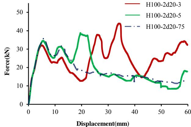
Fig. 8 Load-displacement curves for three specimens with different cutout position from the experiments
