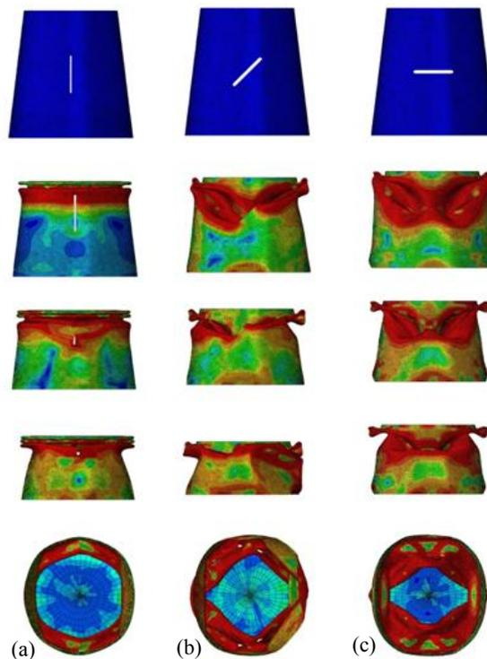
Fig. 4 Shell deformation during crashing phenomena for specimen (a) H70-2-w1-A0, (b) H70-2-w1-A45, (c) H70-2-w1-A90, form FEA.
