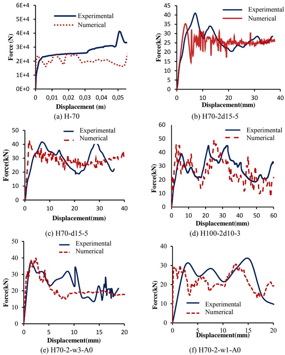
Fig. 5 Comparison of experimental and numerical load–deformation curves of specimen
