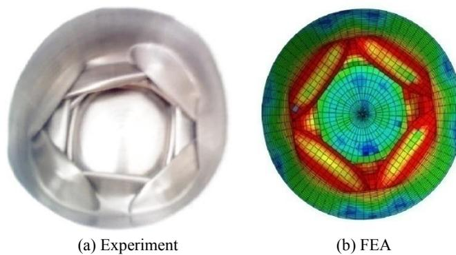
Fig. 6 Collapse mode for specimen H100
