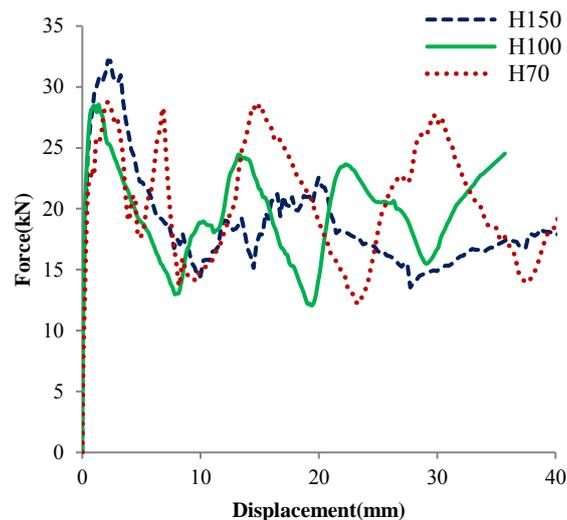
Fig. 7 Load-displacement curves for three specimens with different height from the FEA
