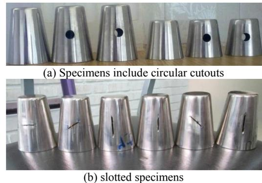
Fig. 1 specimens before test
