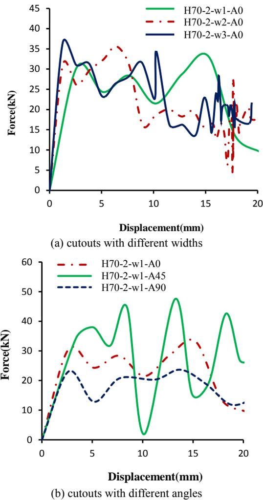
Fig. 9 Load-displacement curves for three specimens containing cutouts from the experiments
