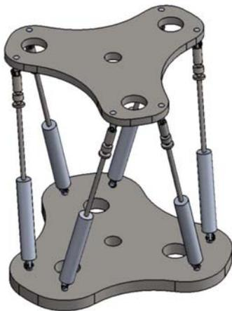
Fig 1: Stewart Platform Mechanism
