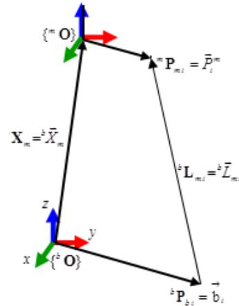
Fig 2: Coordinate axis used in Stewart platform analysis
