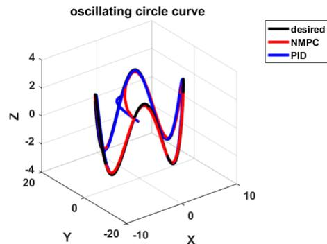
Fig 8: Results of comparison of the NMPC and PID controllers for Circle Oscillating Curve
