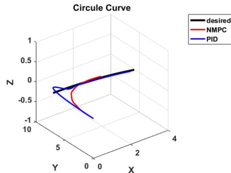
Fig 7: Compare NMPC with PID controller in first 0.5 second
