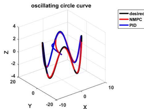
Fig 8: Results of comparison of the NMPC and PID controllers for Circle Oscillating Curve
