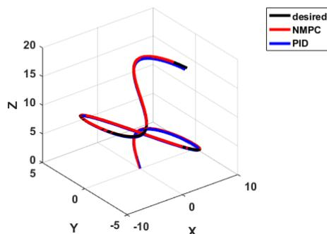
Fig 11: Results of comparison of the NMPC and PID controllers for Eight Oscillating Curve
