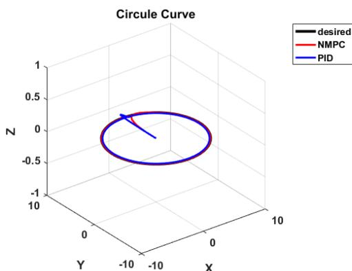
Fig 6: Results of comparison of the NMPC and PID controllers for Circle Curve
