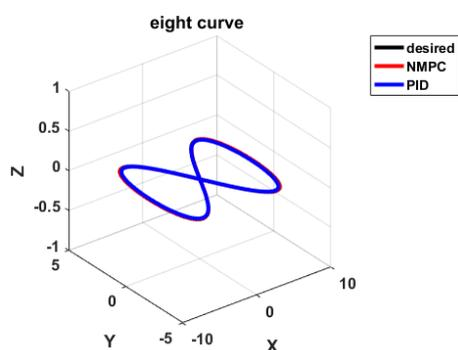
Fig 10: Results of comparison of the NMPC and PID controllers for Eight Curve
