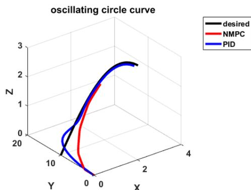
Fig 9: Compare NMPC with PID controller in first 0.4 second
