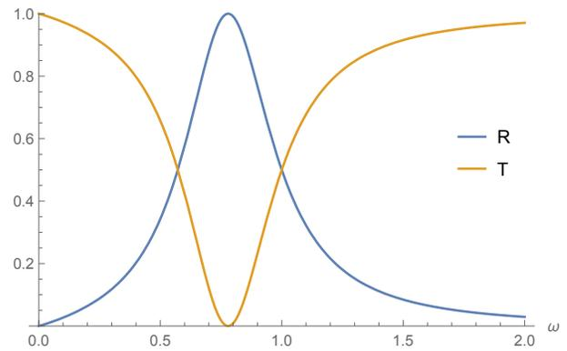
Figure 5: Reflection and Transmission coefficients with the following numerical characterization,  $K_M = 0.1, \rho = 1, m = 1, k = 1$ .
