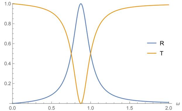
Figure 2: Reflection and Transmission coefficients with the following numerical characterization,  $K_M = 1, \rho = 1, m = 1, k = 1$ .
