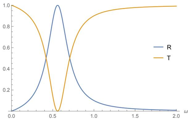
Figure 4: Reflection and Transmission coefficients with the following numerical characterization,  $K_M = 1, \rho = 1, m = 2, k = 1$ .
