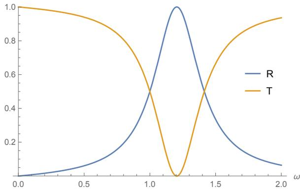
Figure 3: Reflection and Transmission coefficients with the following numerical characterization,  $K_M = 1, \rho = 1, m = 1, k = 2$ .
