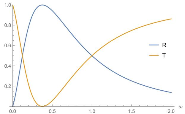
Figure 6: Reflection and Transmission coefficients with the following numerical characterization,  $K_M = 1, \rho = 0.1, m = 1, k = 1$ .
