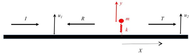
Figure 1: A mass-spring system with rigidity  $k$  and mass  $m$  inside an indefinite beam at the position  $X = 0$ . Incident, reflection and transmission coefficients are made explicit.
