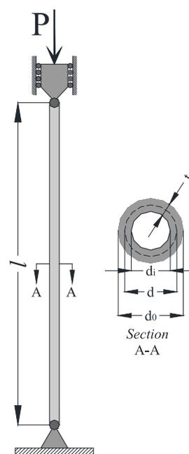
Figure 1. Tubular column and A-A cross-section
