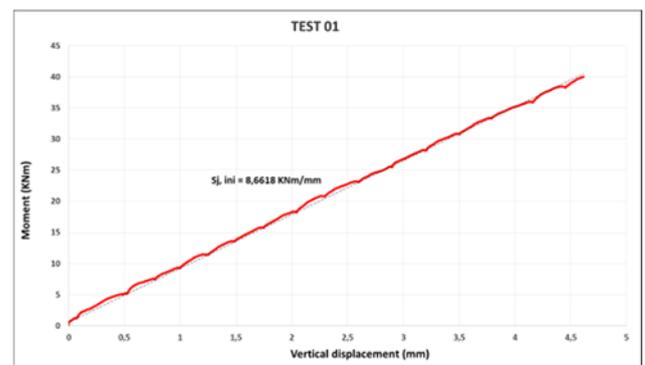
Figure 5. Moment-Displacement diagram for major axis with no loading in the minor axis
