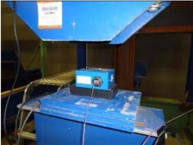
Figure 1. Detail of the displacement sensors
