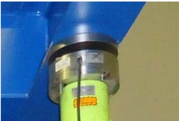
Figure 2. Detail of the load cells
