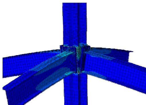
Figure 7. Complete FEM of the joint
