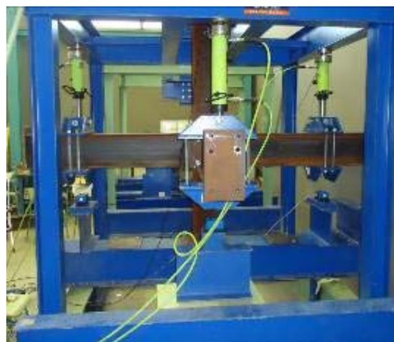
Figure 2. Test arrangement of the external joint.
