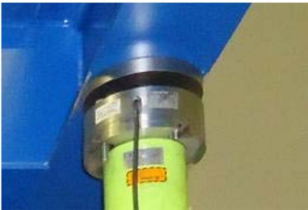
Figure 2. Detail of the load cells
