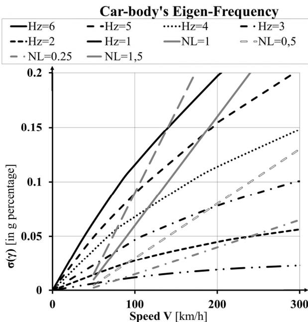
Fig. 4 Comparison of (1) the measured values of the standard deviation of the vertical accelerations  $\sigma(\gamma)$  [of railway vehicles] in relation to the running speed and the eigenfrequencies of the railway vehicles (see [8], [13]) and (2) the values of the empiric Eqn (18) for four values of the coefficient  $N_L=0.25, 0.50, 1.00$  and  $1.50$ .
