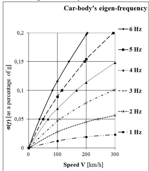
Fig. 3 Measured values of the standard deviation of the vertical accelerations  $\sigma(\gamma)$  [of railway vehicles] in relation to the running speed and the eigenfrequencies of the railway vehicles (see [8], [13], [12]).
