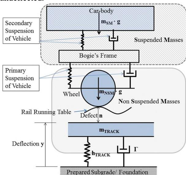
Fig. 2 Model of a Vehicle running the Rail Running Table; the Non-Suspended Masses (NSM) and the Suspended Masses (SM), the primary and secondary suspensions are depicted.
