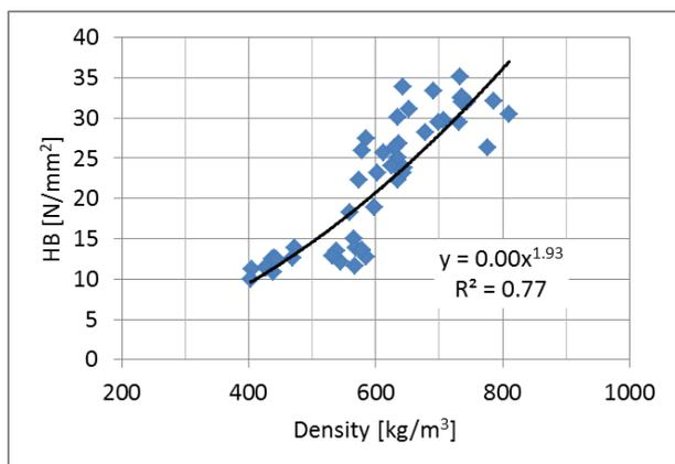
Figure 3 Dependence of Brinell hardness of wood and density of wood floorings
