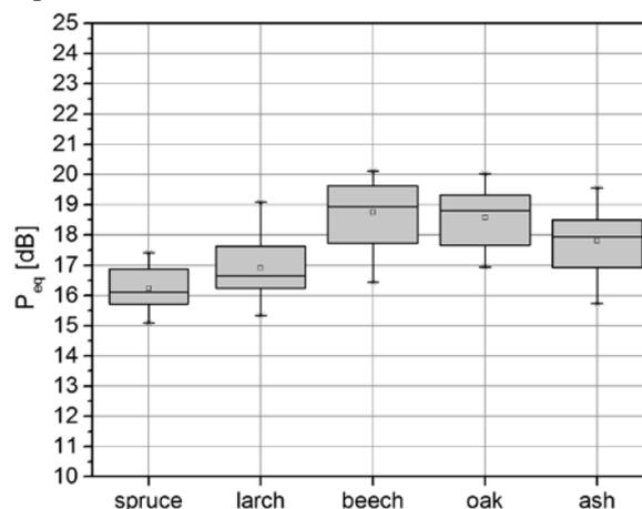
Figure 5 The emitted average sound pressure at testing of different wooden floorings
