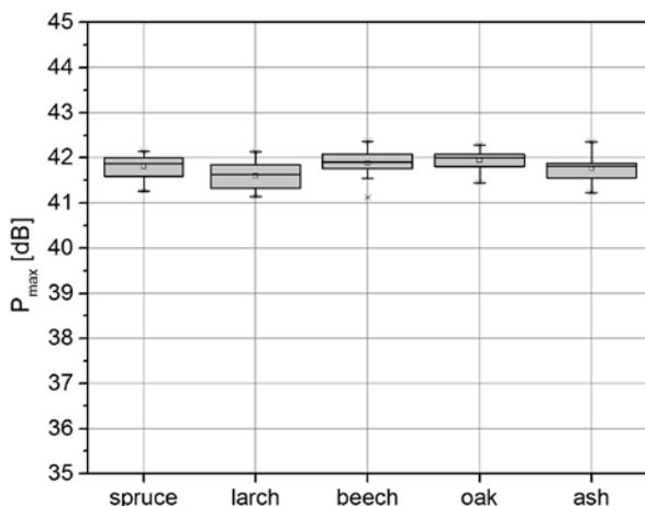
Figure 4 The emitted maximum sound pressure at testing of different wooden floorings
