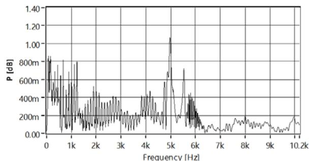
Figure 8 Frequency spectrum of emitted sound at spruce flooring
