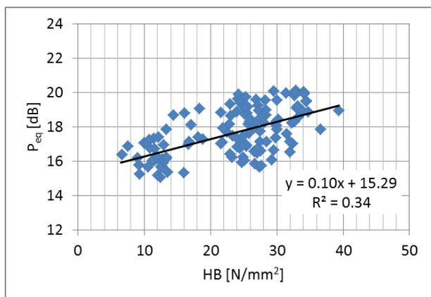
Figure 6 The relationship between average sound pressure and Brinell hardness of tested wooden floorings
