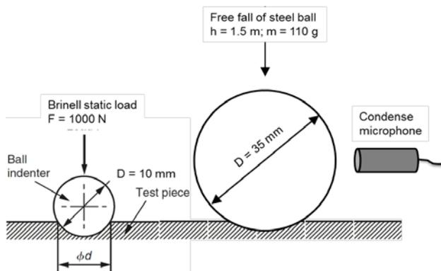
Figure 1 Experimentation setup for Brinell hardness (left) and dynamic impact resistance determination (right)
