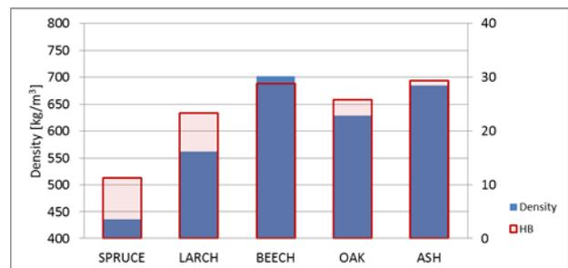
Figure 2 The trend of mean Brinell hardness and density of tested wood species
