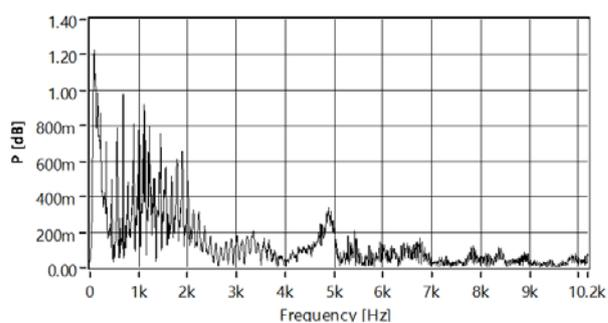
Figure 9 Frequency spectrum of emitted sound at beech flooring
