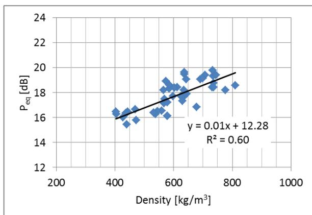
Figure 7 The relationship between average sound pressure and density of tested wooden floorings
