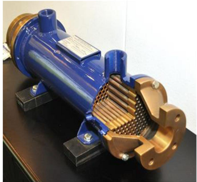
Figure 1. Sketch of segmental cut of semi-industrial prototype of a shell and tube exchanger
