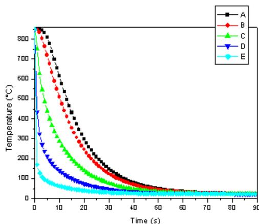
Fig. 3. Temperature profiles on water quenching of C32 steel
