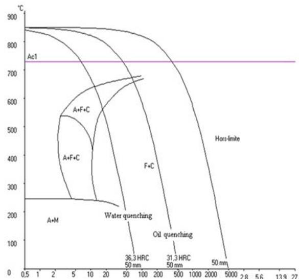
Fig. 2. Cooling curves of C70 steel by water and oil shown on a TTT diagram
