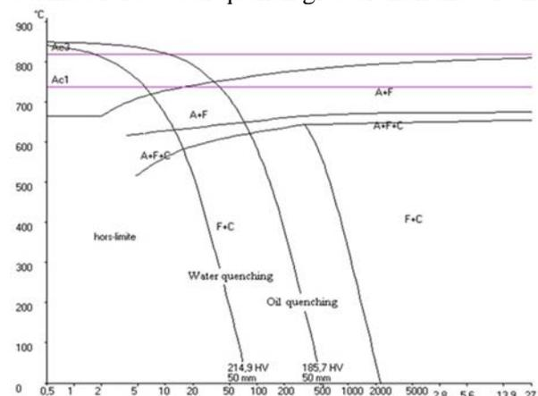
Fig. 1. Cooling curves of C32 steel by water and oil shown on a TTT diagram
