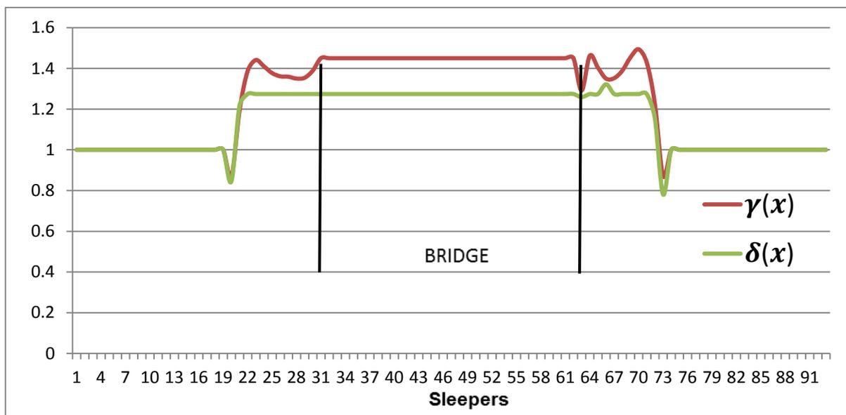
Figure 12: The optimal controlling functions in case of less rigid superstructure
