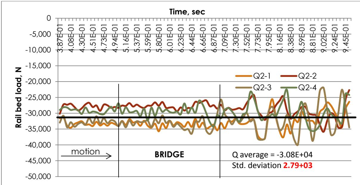
Figure 7: Rail bed load before optimization (perspective train)
