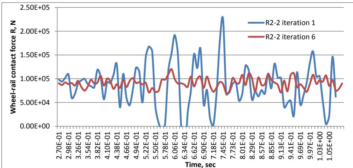
Figure 3: An example of vertical wheel-rail contact force before and after optimization.
