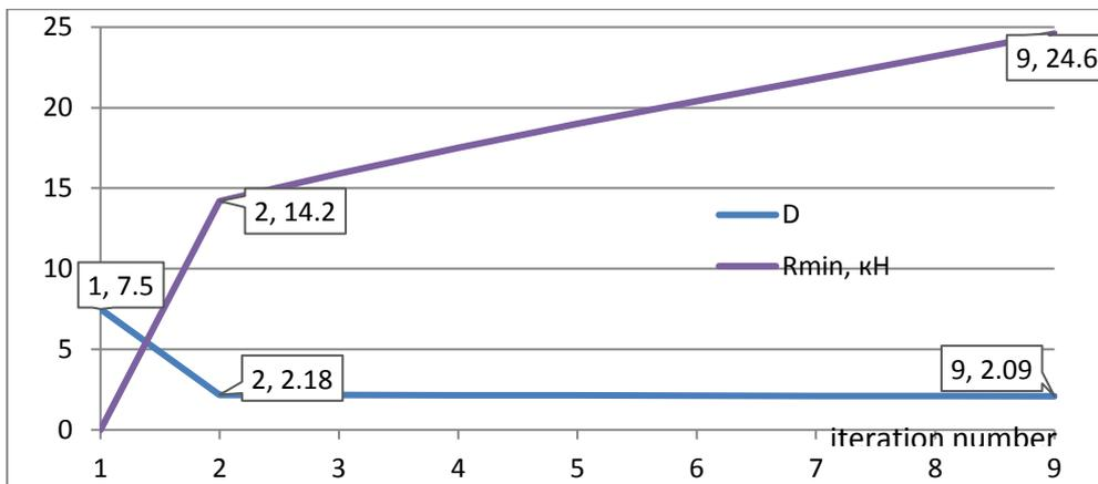
Figure 6: Vertical minimal wheel-rail contact force  $R_{min}$  and  $D$  criterion
