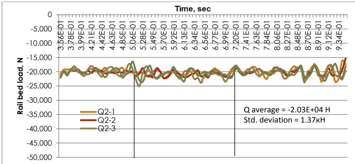
Figure 9: Rail bed load under the second car of CHR380 train after track optimization for perspective train
