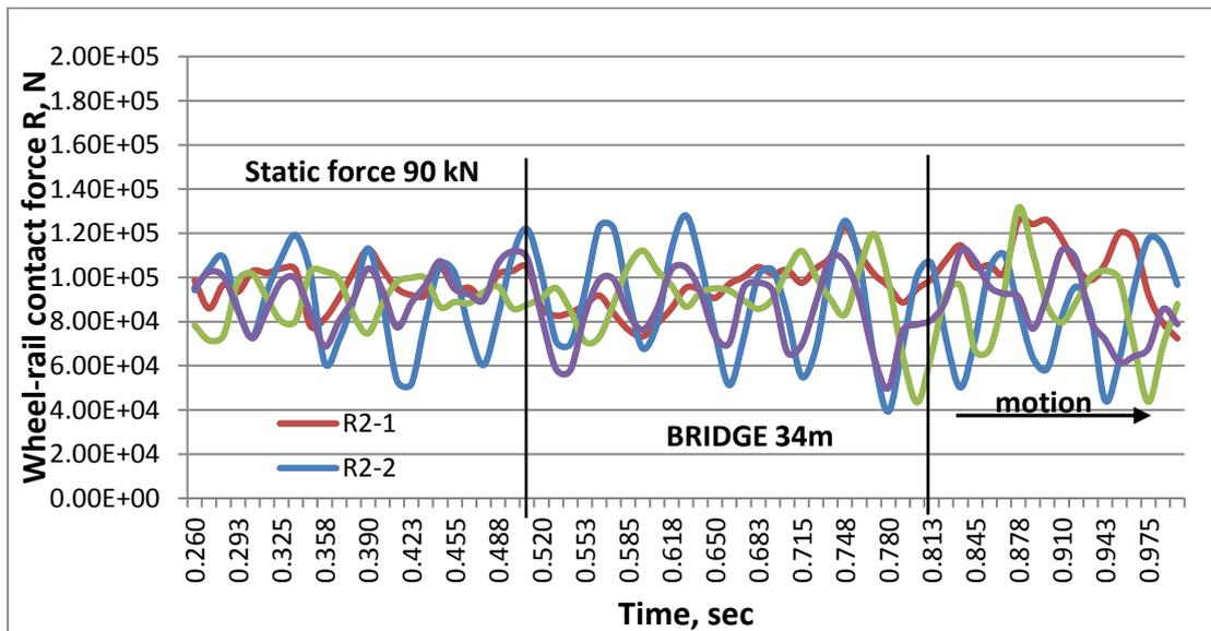
Figure 5: Vertical forces of four wheels of the car of a train during motion through the bridge after optimization
