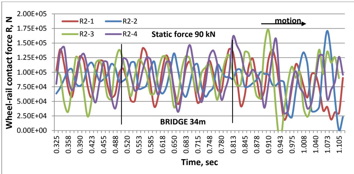
Figure 4: Vertical forces of four wheels of the car of a train during motion through the bridge before optimization
