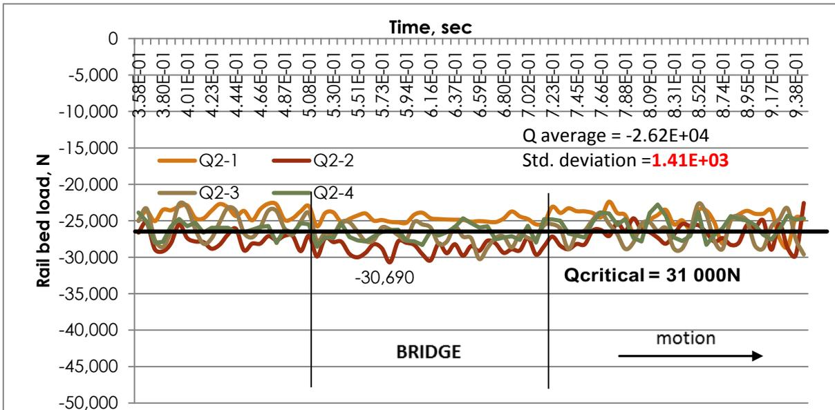
Figure 8: Rail bed load after optimization (perspective train)
