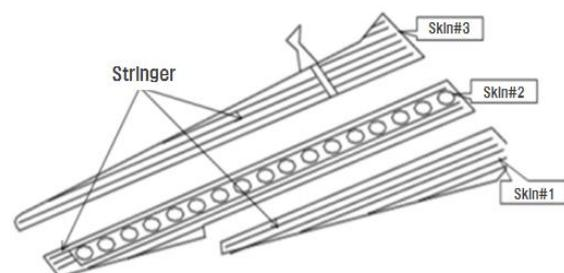
Fig. 1 Arrangement of the stringers
