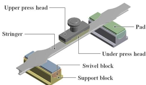
Fig. 3 3D model of the forming system
