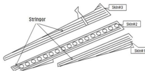
Fig. 1 Arrangement of the stringers
