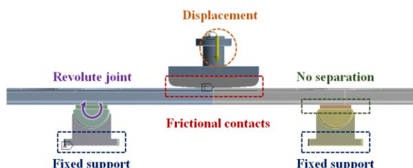
Fig. 4 Boundary conditions of the plastic analysis
