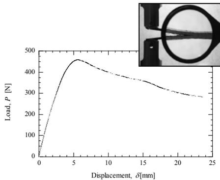
**Fig.2** Load–displacement curve in unidirectional commingled CF/PA12 laminates.
