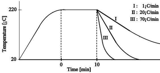
**Fig.1.** Schematic representation of the different thermal conditions applied during processing of commingled CF/PA12 composites.
