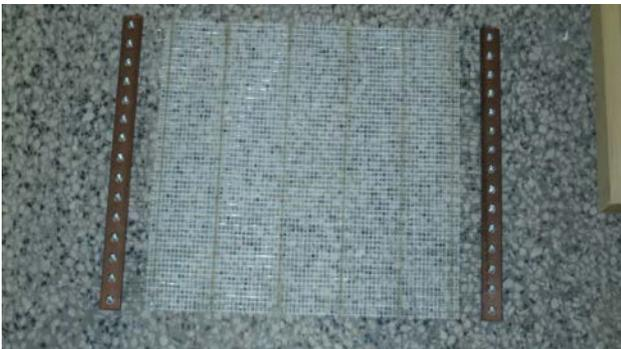
Fig. 6: Electric resistance wire prepared on plastic netting
