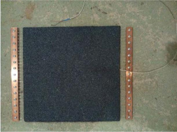
Fig. 5: Electric resistance wire between two layers of asphalt belt
