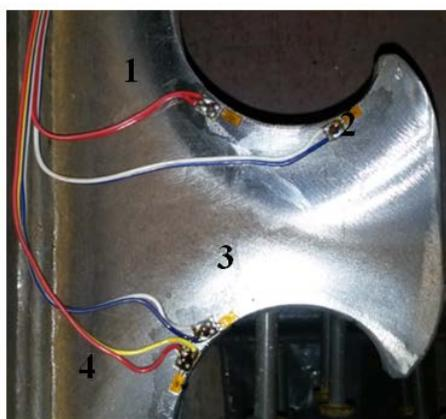
Figure 6: The positions of strain gauges
