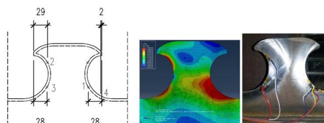
Figure 4: Identification of HOT SPOT, strain gauges
