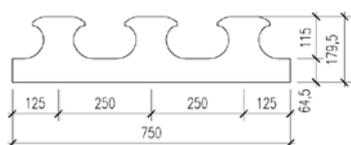
Figure 2: The diameters of the steel strip
