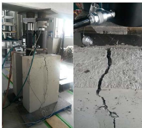
Figure 7: Failure of the test specimen V9
