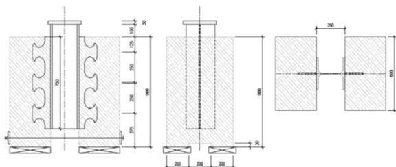
Figure 1: Push-out test scheme
