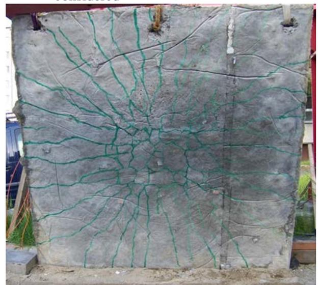
Fig. 11 Cracks on the bottom surface of the slab
