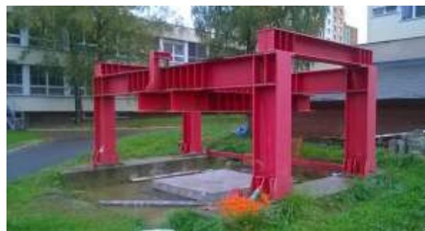
Fig. 1: Testing devise – steel frame structure
