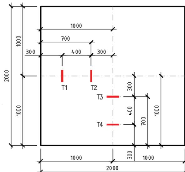
Fig. 4: Scheme of strain gauges position
