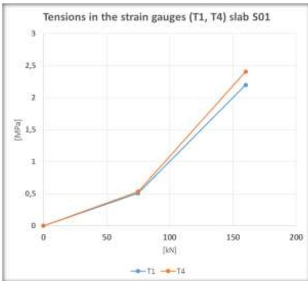
Fig.6: S01- tensions in the strain gauges T1, T4
