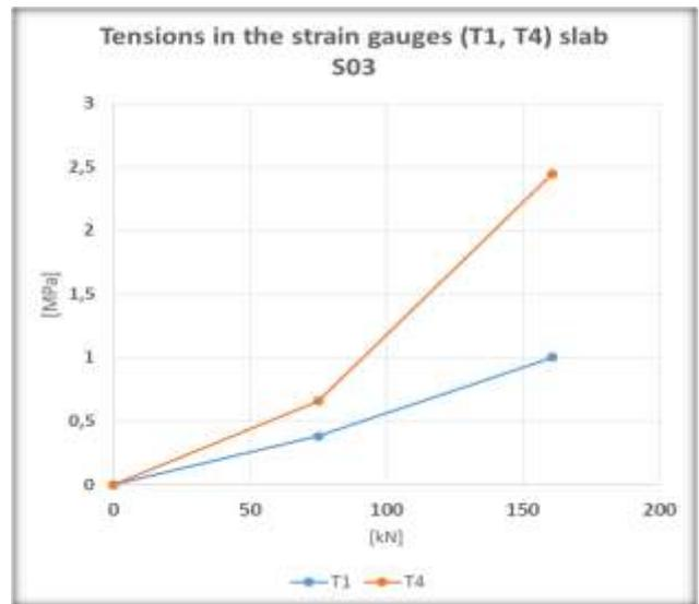
Fig.10: S03 - tensions in the strain gauges T1, T4
