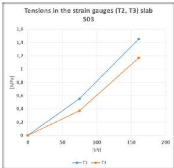
Fig.11: S03 - tensions in the strain gauges T2, T3
