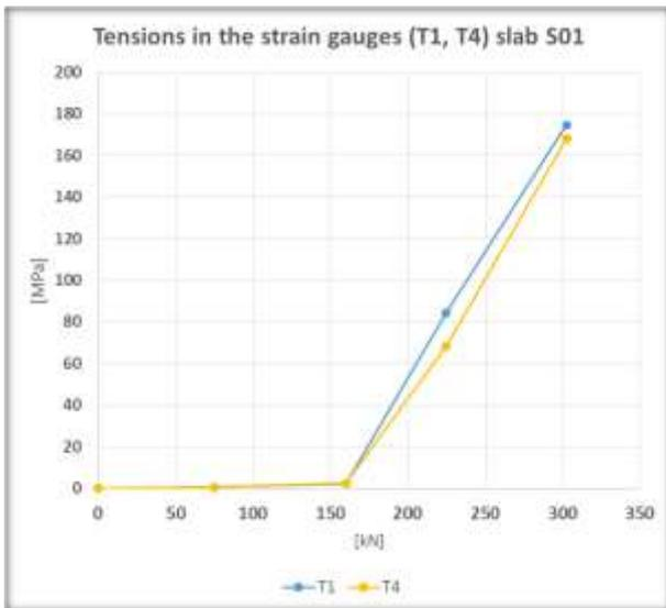
Fig.5: S01 - tensions in the strain gauges T1, T4
