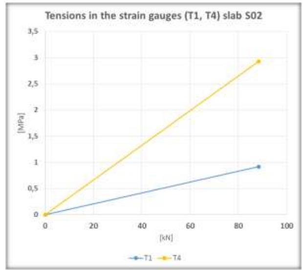
Fig.9: S02 - tensions in the strain gauges T1, T4
