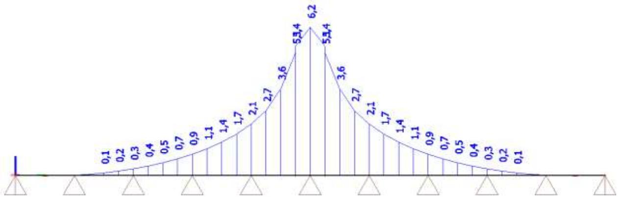
Fig. 13: Tension [MPa] in slab foundation by FEM analysis. Load of 75kN.
