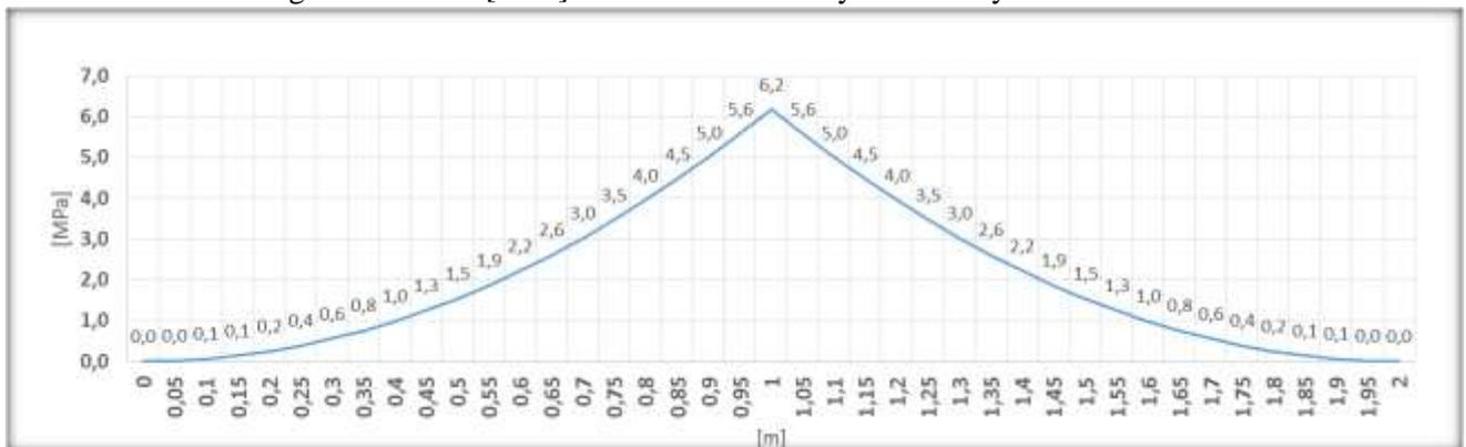
Fig. 14: Tension [MPa] in slab foundation by simplified calculation. Load of 75kN.
