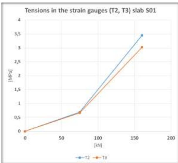
Fig.7: S01- tensions in the strain gauges T2, T3
