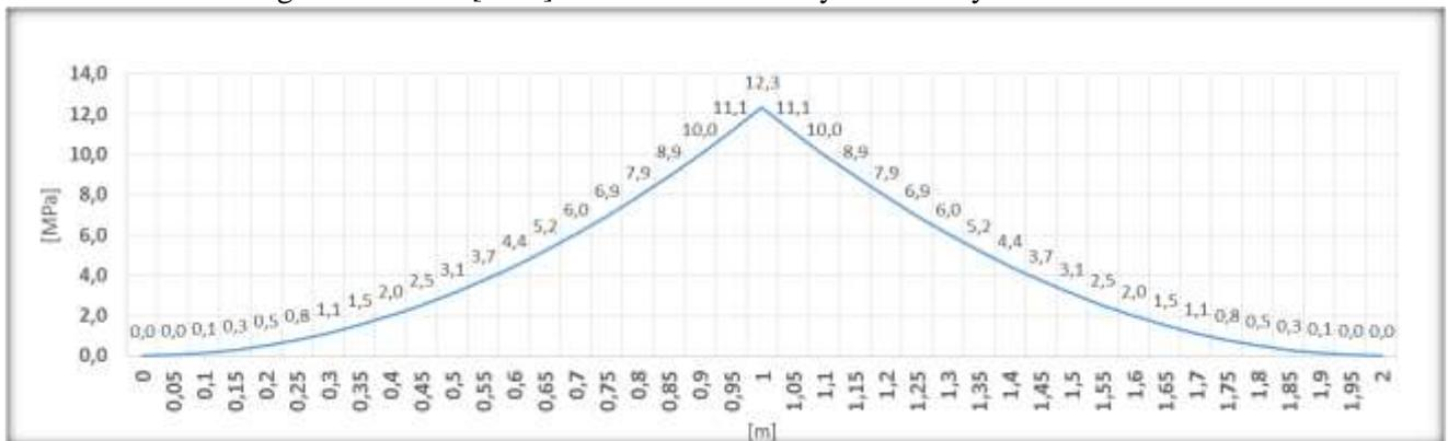
Fig. 16: Tension [MPa] in slab foundation by simplified calculation. Load of 150kN.
