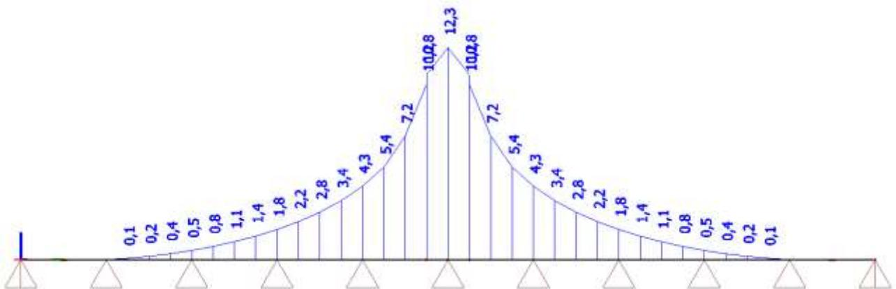
Fig. 15: Tension [MPa] in slab foundation by FEM analysis. Load of 150kN.
