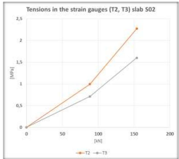
Fig.8: S02 - tensions in the strain gauges T2, T3
