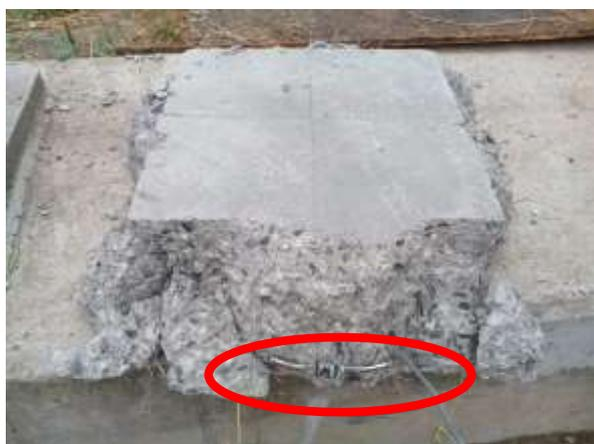
Fig. 12: Damaged gauge after completing the test
