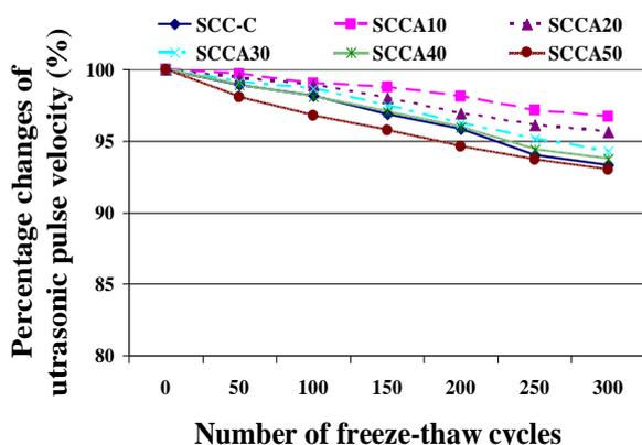
**Fig. 2.** UPV as percentage at every 50 freeze-thaw cycles
