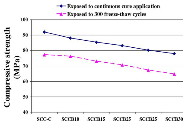
Fig. 5. Compressive strength of specimens
