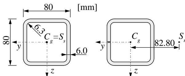
Fig.2: Cross sections: a) hollow, b) open.
