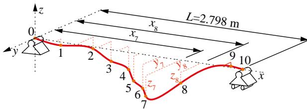
Fig.4: Definition of spatial curvature of the axis.
