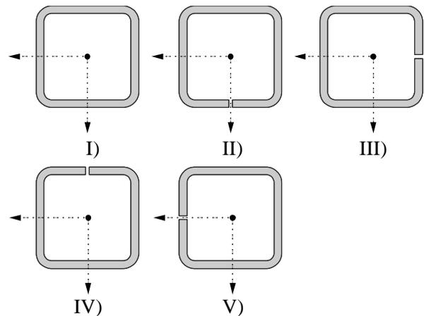
Fig.3: Hollow and open cross sections.
