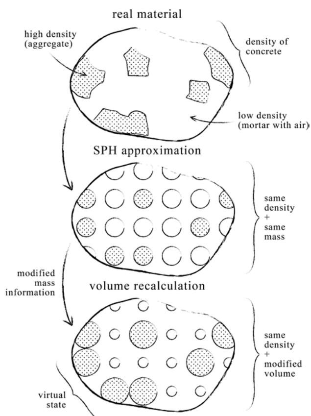
Fig. 3. Including the numerical heterogeneity in the SPH model.
