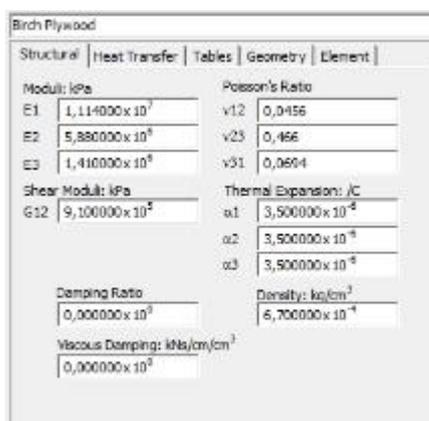
Fig.8 Mechanical characteristics of the wood utilized for the plate elements.
