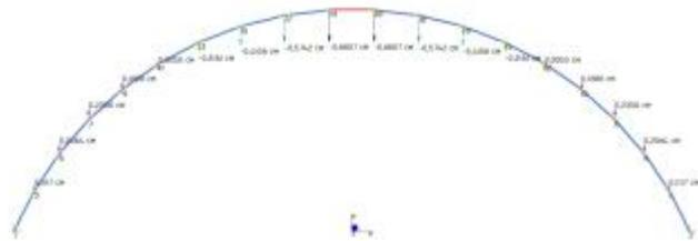
Fig. 6 Lowerings with a load equal to 24 kN
