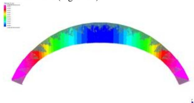
Fig. 10 "Contour" plot of the lowerings
