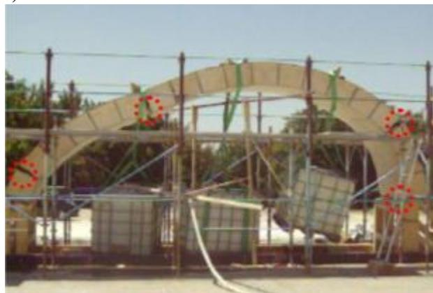
Fig. 2 Tested arch. a) details with the low tanks of the positioning of the displacement transducers; b) collapse mechanism and achievement of the hinges in the arch with an asymmetric load condition.
