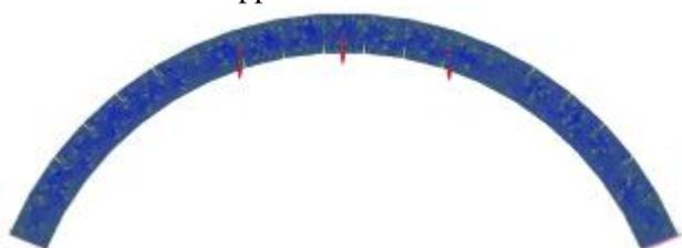
Fig. 7 "Warping" view of the arch with plate elements and applied loads
