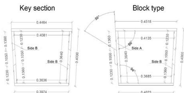
Fig. 1 Executive drawings of the blocks with the connecting system by mean of male-female joints.
