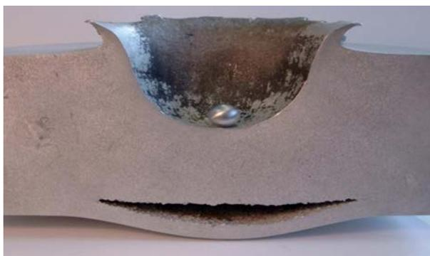
**Figure 14:** A typical thick plate with the crater formed at the top caused by a spherical projectile which is embedded in the bottom of the crater and a single scab detached from the rear end due to the reflected tensile wave.
