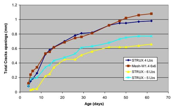
**Fig. 10.** Plot of total crack openings versus time for set one.
