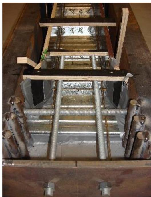
Fig. 1. Details of end restraint.
