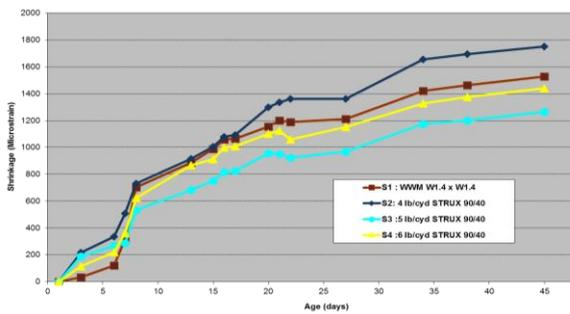
**Fig. 6.** Plot of free shrinkage strain versus time for set two.
