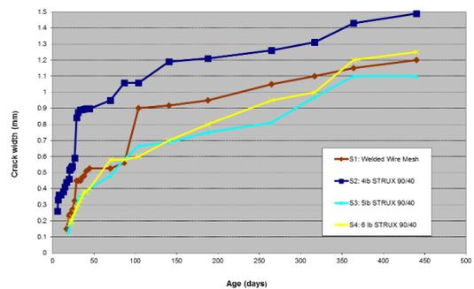
**Fig. 9.** Plot of maximum crack width versus time for set two.
