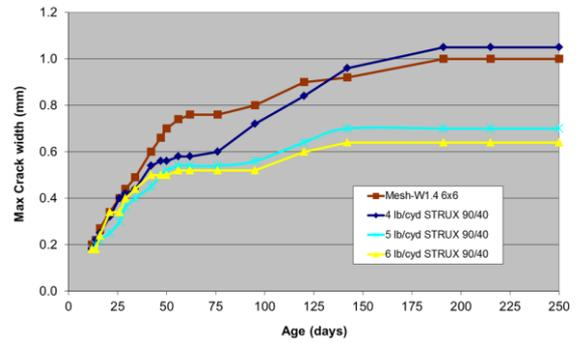
**Fig. 8.** Plot of maximum crack width versus time for set one.
