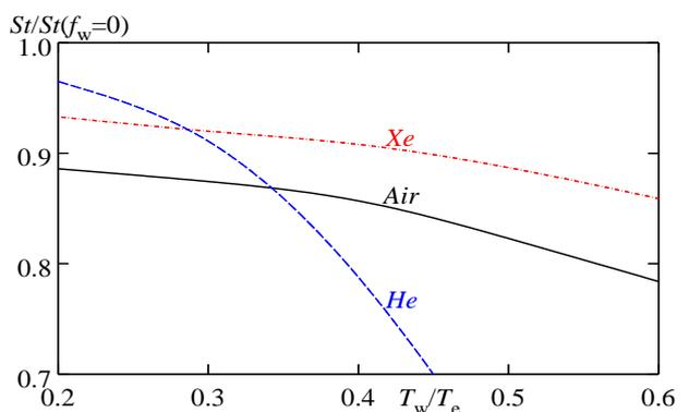
Fig.4: Influence of the wall temperature on Stanton number at  $M=0.7$ .
