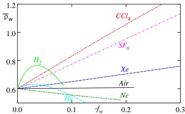
Fig.6: Density of the mixture at the wall  $\bar{\rho}_w$  versus injection factor  $-f_w$ .
