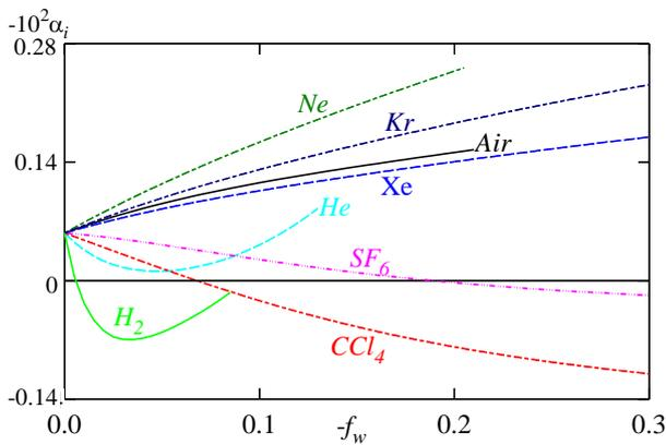
Fig.5: Spatial amplification rate  $-\alpha_i$  versus injection factor  $-f_w$  for variety of foreign gases;  $Re = 720, F \cdot 10^6 = 35$ .
