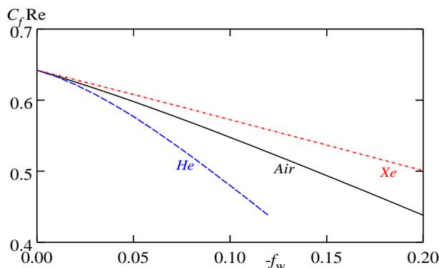
Fig.2: Normalized skin friction coefficient  $C_f Re$  versus injection factor for the adiabatic wall;  $M=2$ .
