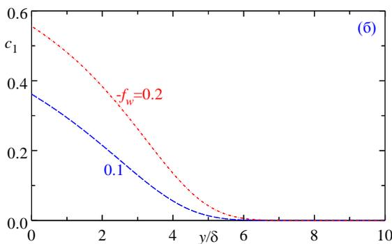
Fig.1: Distribution of the mass concentration of  $CCl_4$  across the boundary layer for two values of  $-f_w$ .
