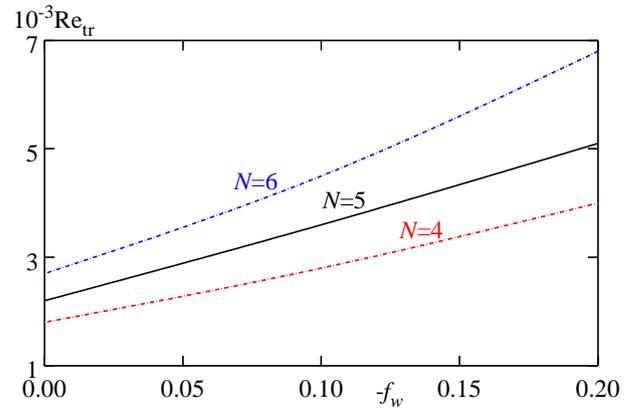
Fig.7: Transition Reynolds number  $Re_{tr}$  versus injection factor  $-f_w$  for  $CCl_4$ , as calculated by the  $e^N$ -method;  $M = 2$ .
