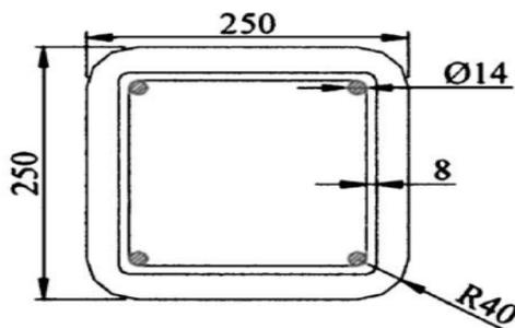
**Fig 2.** Cross-section and reinforcement detail of specimen
