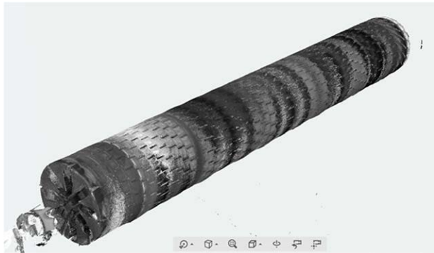
Fig. 4. Point cloud filtered and registered (more than 4 million points).
