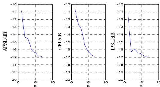
Fig.4 APSL, CPL and IPSL versus the number of quantization bits  $B$
