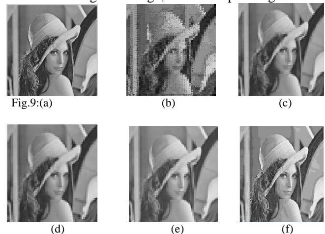
Figure 9: (a) Original lena image (b) Reconstructed image using DCT (c) Reconstructed image using RLE (d) Reconstructed image using Huffmans (e) Reconstructed image using wavelet dB2 filter (f) Reconstructed image using proposed method.
