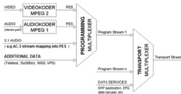
Fig.4 Multiplexer into stream
