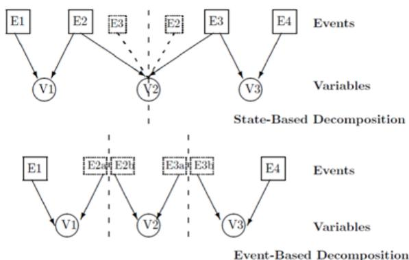
Fig.1 Comparing Event-Based and State-Based Decomposition
