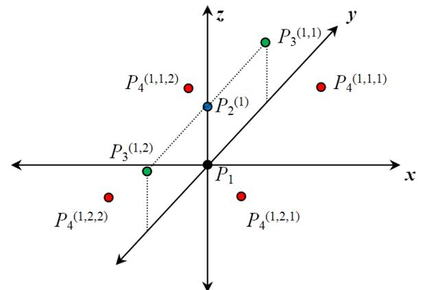
Fig. 2. The four solutions of placing  $P_2$  a distance  $+r_{1,2}$  from the origin on the  $y$ -axis for  $N = 4$ . (i) Two solutions for  $P_3^{(1,1)} = (0,y_3,z_3) = (0, y_3,+r_{1,2})$ :  $P_4^{(1,1,1)}$  and  $P_4^{(1,1,2)}$ . (ii) Two solutions for  $P_3^{(1,1)} = (0,y_3,z_3) = (0, -y_3,+r_{1,2})$ :  $P_4^{(1,2,1)}$  and  $P_4^{(1,2,2)}$ .
