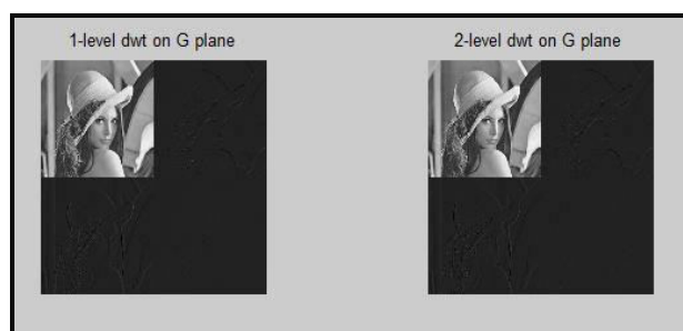
Fig. 6 Application of the 2-level DWT on the G plane of the RGB cover image
