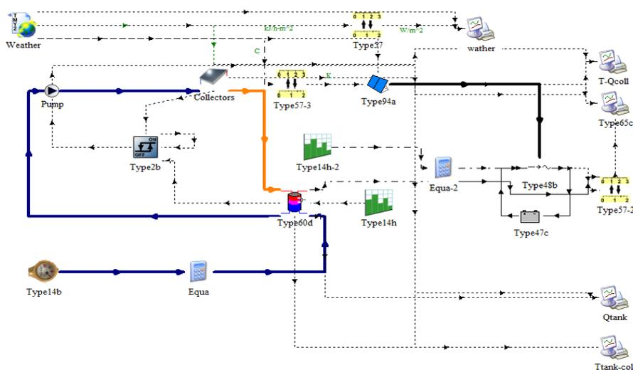
**Fig.6 The model that combines the thermal system for the distillation membrane and the photovoltaic system.**
