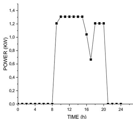
**Fig.8 Outlet Temperature of Storage Tank. Fig.9 Power load of the photovoltaic system**
