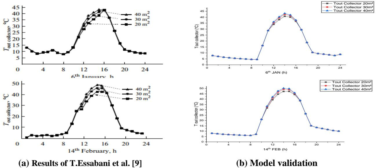
**Fig.5 Variation of collector outlet temperature as function of collector area.**
