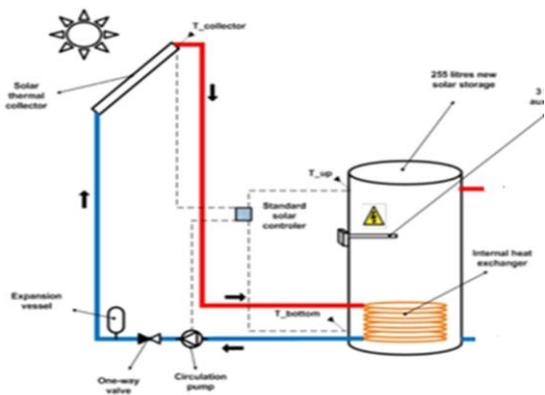
Fig. 1 solar hot water system.
