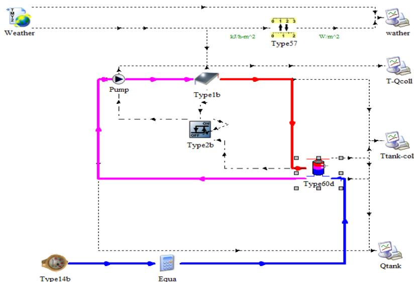
Fig.3 Assembly diagram of the solar system in the TRNSYS simulation.
