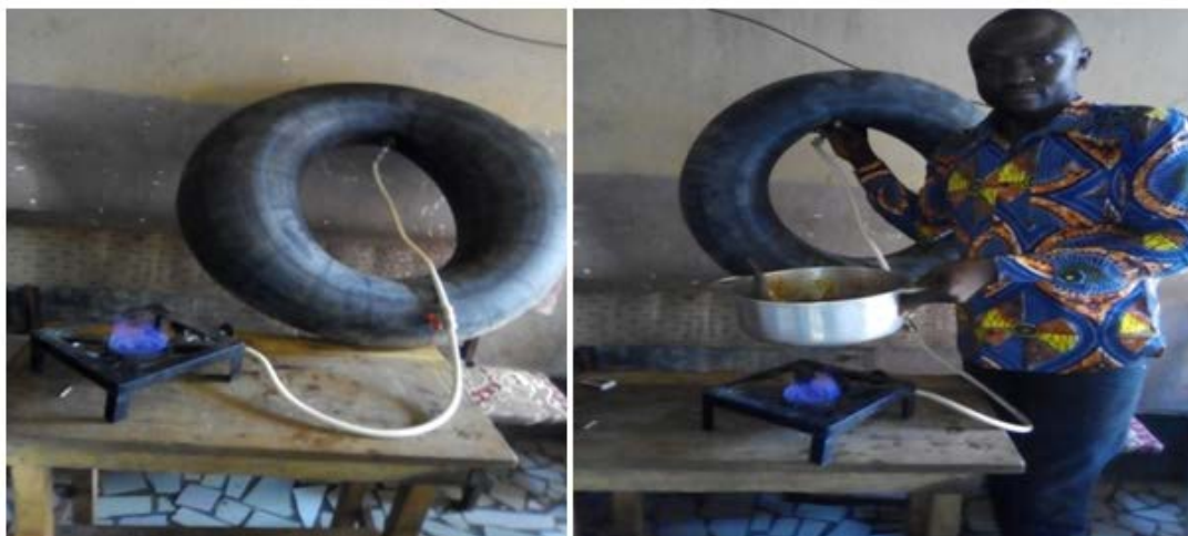
Photo 11: Biogas combustion test
