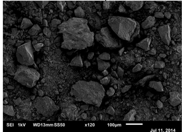
Figure 4: Microstructure of Coal
