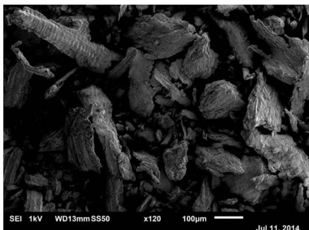
Figure 6: Microstructure of Torrefied Wood Pellet
