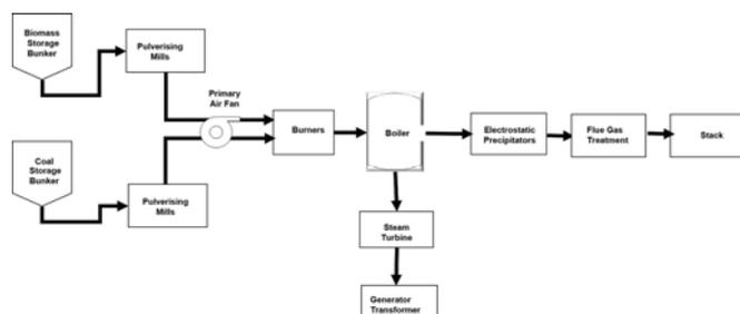
Figure 7: Direct Co-Firing Biomass-Coal Power Plant Outline
