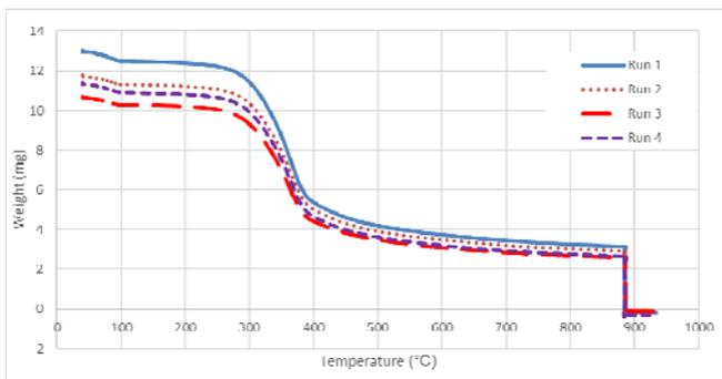
Figure 3: TGA Graphs Torrefied Wood Pellets
