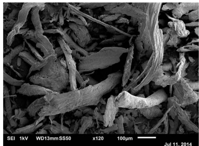
Figure 5: Microstructure of Wood Pellet
