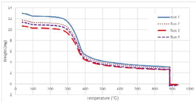
Figure 3: TGA Graphs Torrefied Wood Pellets
