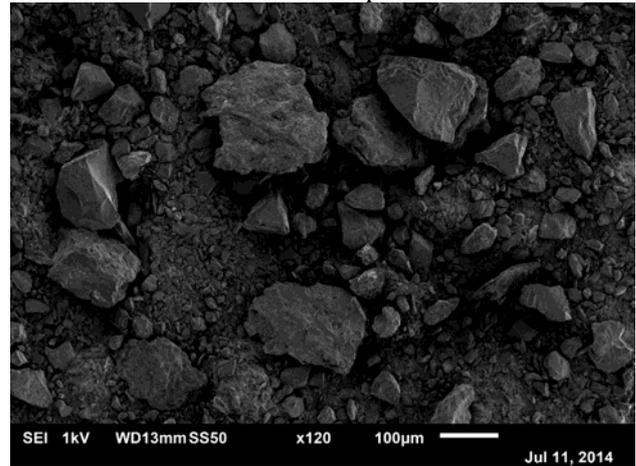
Figure 4: Microstructure of Coal
