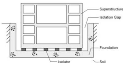
Fig.9: Components of a Base Seismic Isolated Structure, [16].
