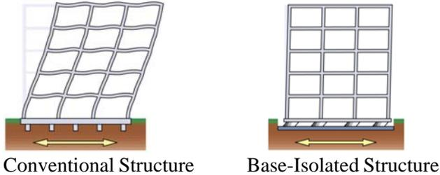
Fig.7: Comparison of Conventional and Base-Isolated Structures showing Laterally Flexible Layer between Structure and Foundation, [15].
