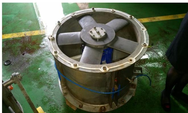
Fig. 2. Wells turbine for the Mutriku OWC wave power plant
