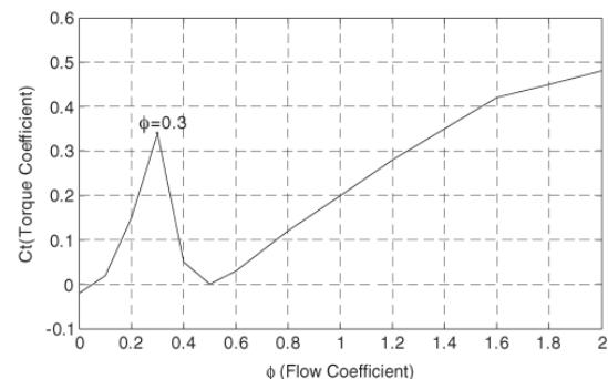
Fig. 4. Torque Coefficient vs. Flow Coefficient
