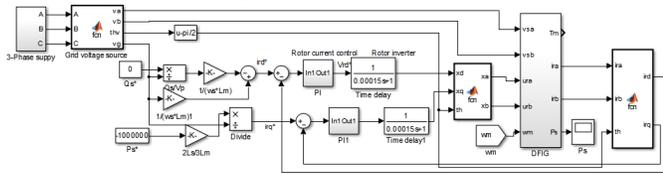
Figure11. DFIG Modeling for  $P_s$  &  $Q_s$  control
