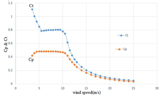
Figure 2.  $C_p$  &  $C_t$  versus wind speed curve of DFIG
