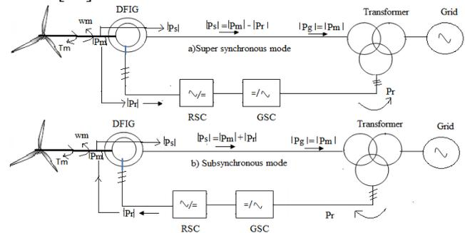
Figure 3 Power flow in DFIG WECS
