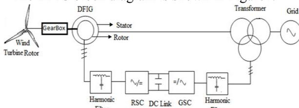
Figure1. Simplified block diagram for DFIG WECS.
