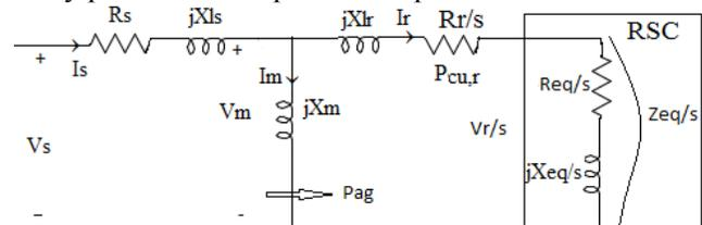
Figure 4. Steady-state equivalent circuit of DFIG with the RSC represented by  $R_{eq}$  and  $X_{eq}$
