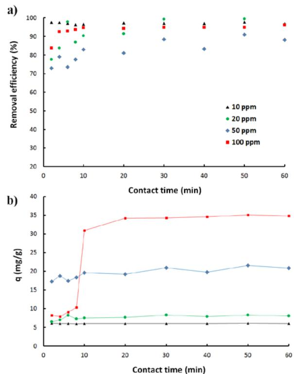
Fig. 6. Influence of contact time on the  $Pb^{2+}$  removal efficiency (a) and lead uptake (b).
