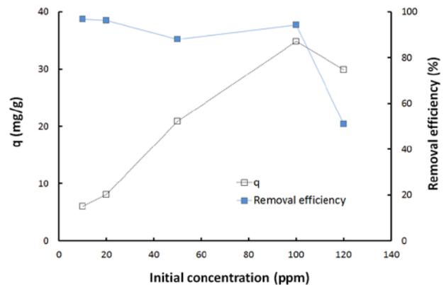
Fig. 3. Effect of initial concentration of Pb<sup>2+</sup> on the removal efficiency of this heavy metal (geopolymer dosage: 0.10 g, pH = 5; contact time: 60 min).
