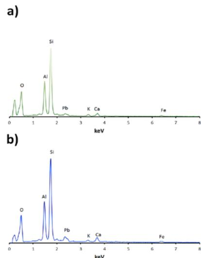
Fig. 4. EDS spectrum of the FA-based geopolymer after 10 min contact time in distinct Pb<sup>2+</sup> concentration: a) 50 ppm and b) 100 ppm.
