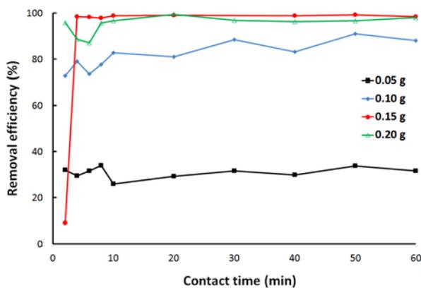
Fig. 5. Effect of geopolymer dosage on the lead removal efficiency ( $[Pb^{2+}] = 50$  ppm, pH = 5).
