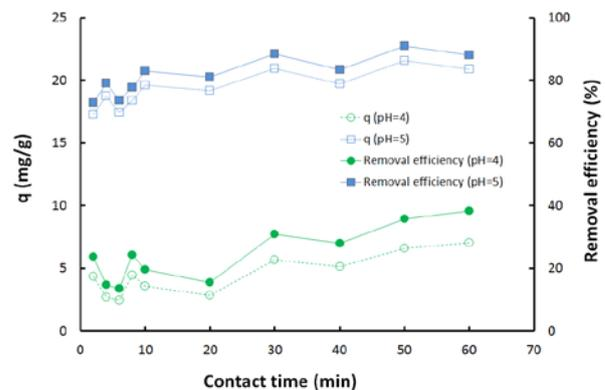
Fig. 7. Influence of pH on the  $Pb^{2+}$  uptake and removal efficiency ( $[Pb^{2+}] = 50$  ppm, geopolymer dosage: 0.10 g).
