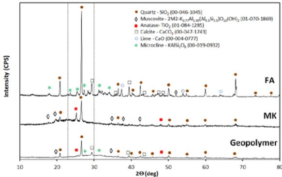
Fig. 1. XRD patterns of FA, MK and the synthesized geopolymer.
