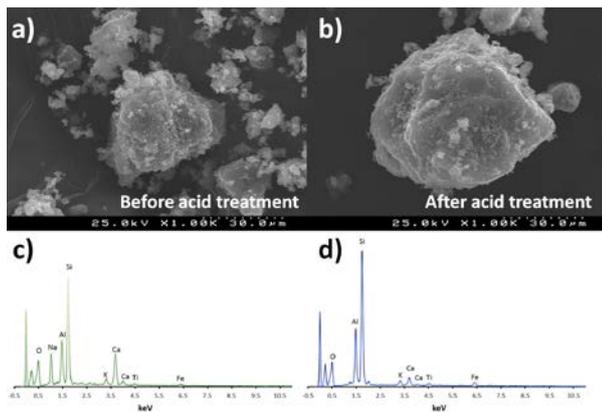
Fig. 2. SEM micrographs (a and b) and EDS spectrum (c and d) of the FA-based geopolymer before (a and c) and after (b and d) acid treatment.
