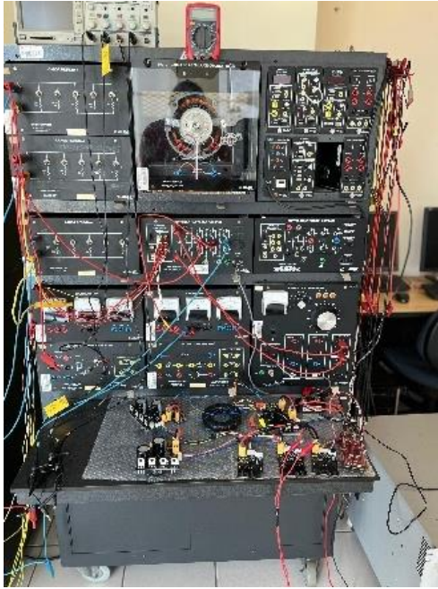
Fig. 7: Overview of the complete experimental setup, including the programmable power source, measurement instruments, and load banks.
