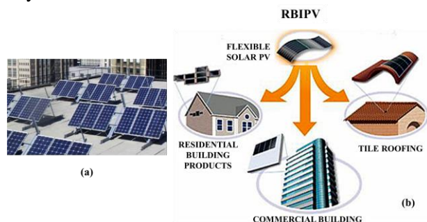
Fig. 3 (a) Traditional SPV rooftop installations, (b) RBIPV installation scheme using flexible PV module
