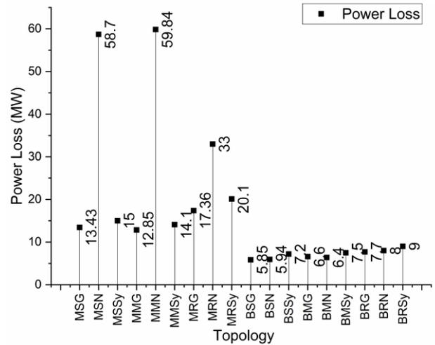
Fig. 16. Overall power loss in Transmission of each topology
