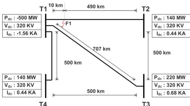
**Fig. 8. Rated load flow at all terminals**
