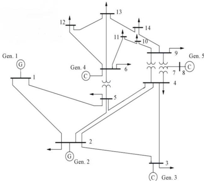
Figure. 1 IEEE 14 bus test system
