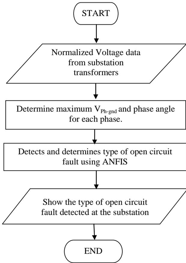
Fig.2: The ANFIS fault detectors flowchart.
