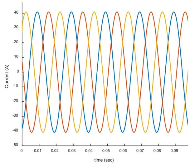
Fig.4: Current waveform during no fault condition.
