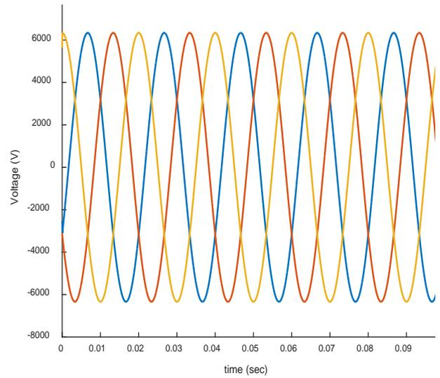
Fig.3: Voltage waveform during no fault condition.
