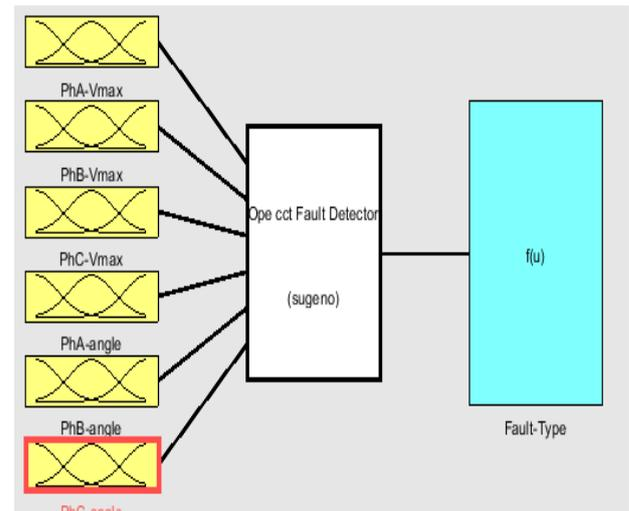
Fig.1: Fuzzy inference system for fault detector and type classifier.
