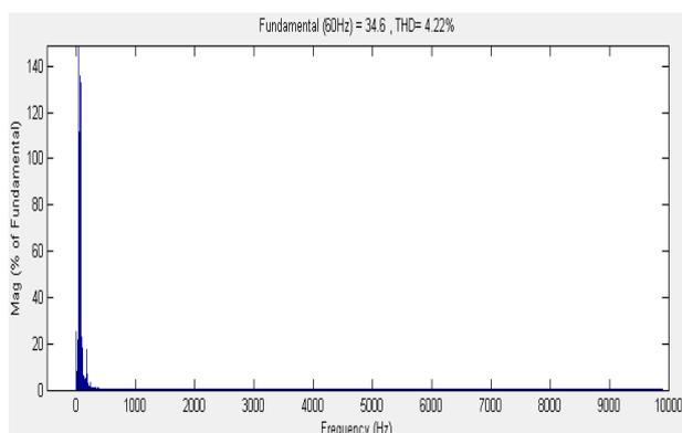
Fig. 8 FFT window for generated current with unbalanced resistive load
