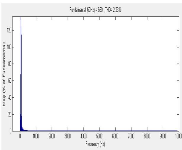
Fig. 5 FFT window for generated voltage with balanced resistive load
