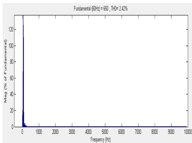
Fig. 7 FFT window for generated voltage with unbalanced resistive load
