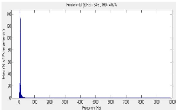
Fig. 13 FFT window for generated current with unbalanced reactive load
