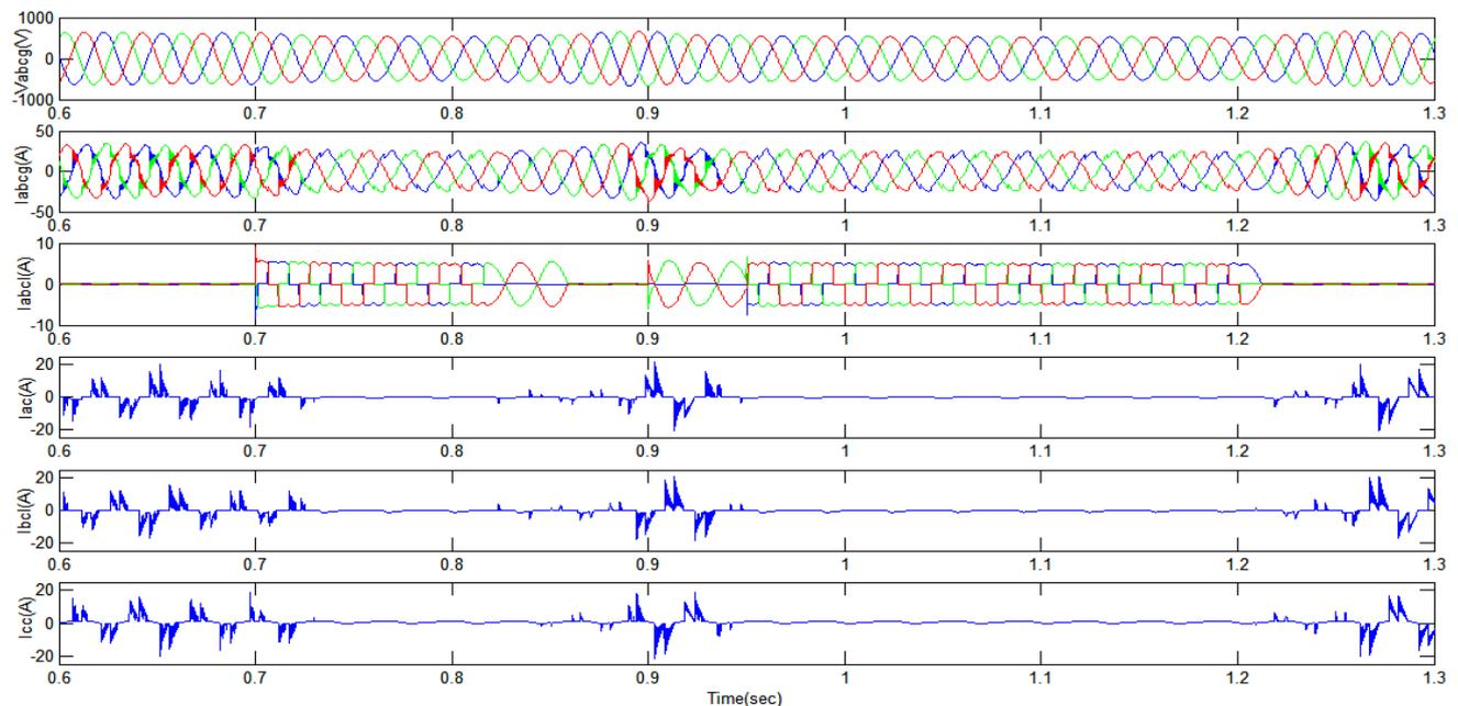
Fig.14 Simulated transient characteristics waveforms of voltage generated by three-phase IAG ( $V_{abcg}$ ), three-phase IAG currents ( $I_{abcg}$ ), three-phase non-linear load currents ( $I_{abcl}$ ), per-phase EVFC currents ( $I_{ac}$ ,  $I_{bc}$ ,  $I_{cc}$ ) under unbalanced non-linear load.
