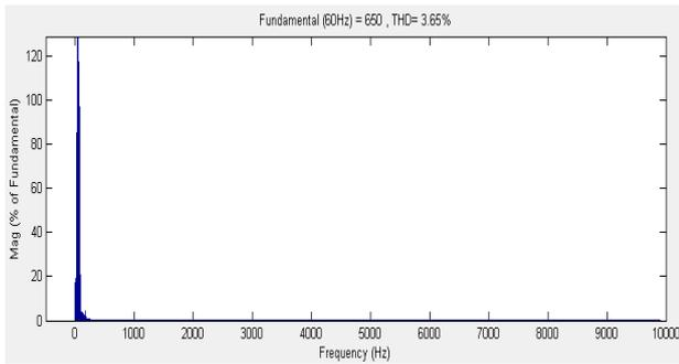
Fig. 15 FFT window for generated voltage with balanced non-linear load
