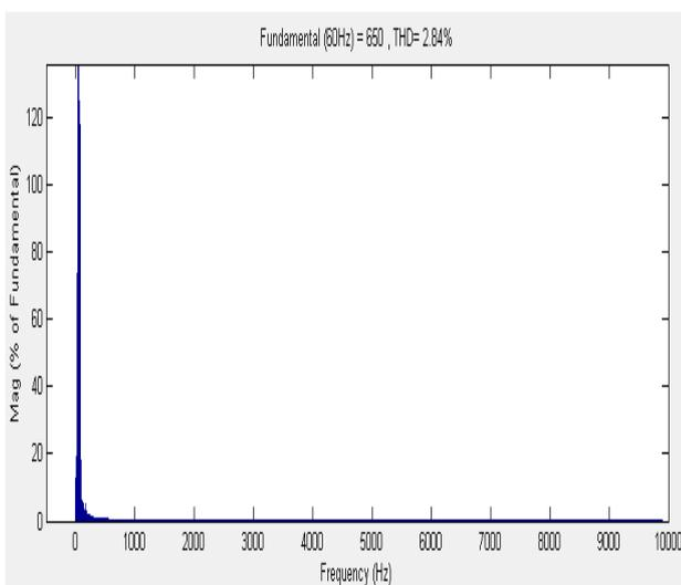
Fig. 10 FFT window for generated voltage with balanced reactive load
