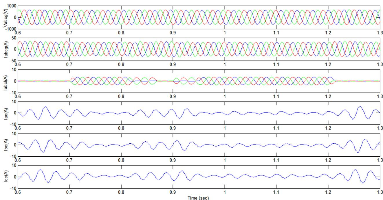
Fig. 2 Simulated transient characteristics waveforms of voltage generated by three-phase IAG ( $V_{abcg}$ ), three-phase IAG currents ( $I_{abcg}$ ), three-phase resistive load currents ( $I_{abcl}$ ), per-phase EVFC currents ( $I_{ac}$ ,  $I_{bc}$ ,  $I_{cc}$ ) under unbalanced resistive load
