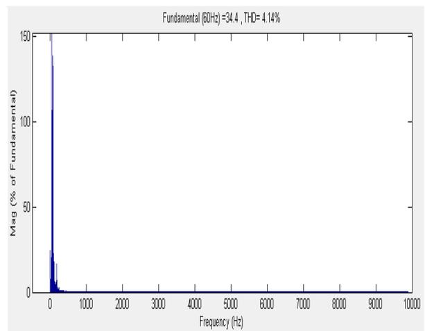
Fig. 6 FFT window for generated current with balanced resistive load
