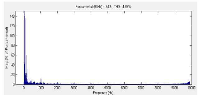
Fig. 18 FFT window for generated current with unbalanced nonlinear load
