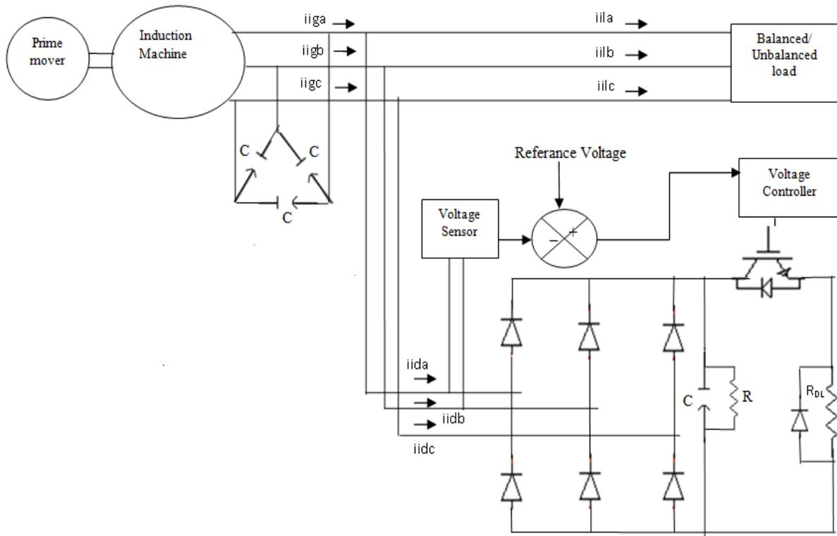
Fig. 1 Simulink model diagram of the whole generating system along with EVFC
