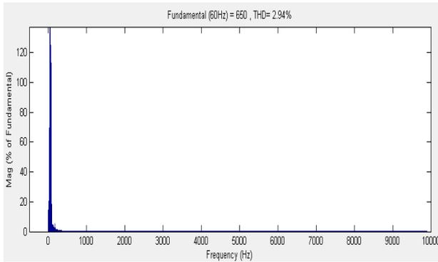
Fig. 12 FFT window for generated voltage with unbalanced reactive load
