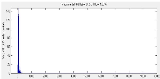
Fig. 16 FFT window for generated current with balanced non-linear load
