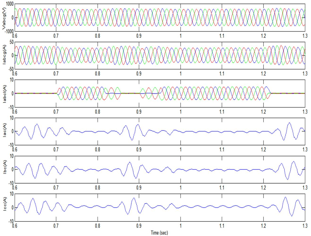
Fig. 9 Simulated transient characteristics waveforms of voltage generated by three-phase IAG ( $V_{abcg}$ ), three-phase IAG currents ( $I_{abcg}$ ), three-phase reactive load currents ( $I_{abcl}$ ), per-phase EVFC currents ( $I_{ac}$ ,  $I_{bc}$ ,  $I_{cc}$ ) under unbalanced reactive load.
