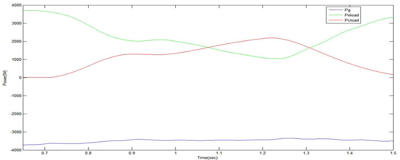
Fig. 4 Variation of power generated by IAG ( $P_{gen}$ ), consumer power ( $P_{cload}$ ) and electronic load power ( $P_{eload}$ ).
