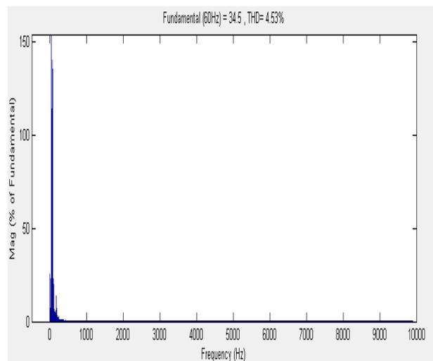
Fig. 11 FFT window for generated current with balanced reactive load
