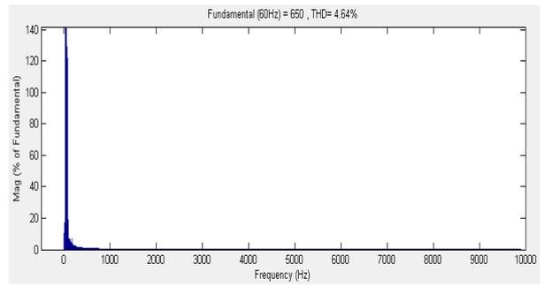
Fig. 17 FFT window for generated voltage with unbalanced non-linear load
