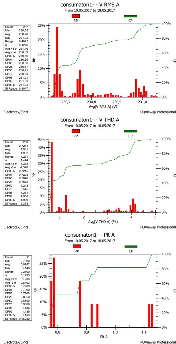
Fig. 4. Histogram of PQ parameters in PoI (4): phase RMS, phase voltage THD, phase Plt
