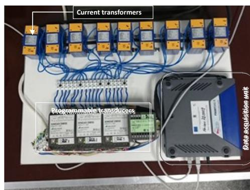
Fig. 3. Connection configuration of the remote data acquisition and transmission units
