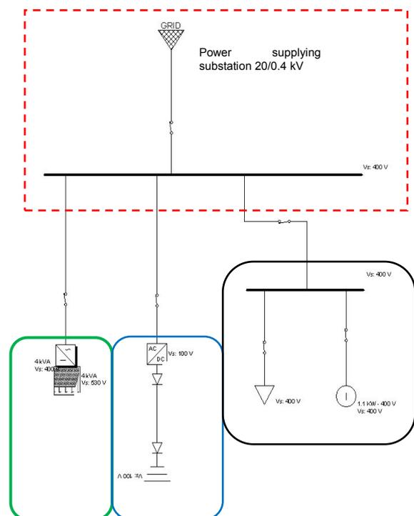
Fig. 1. Configuration of the power supplying network of SGRL
